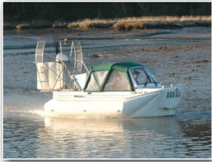
Surveyor-16, our newest craft features a more powerful engine for increased speed, payload and headwind capability. The proven carbon fiber belt drive prevents any slippage, has improved efficiency, requires no re-tensioning, and eliminates the need for belt covers or touch bars, simplifying maintenance. The new idlers feature a double sealed bearing for greatly improved service life over the older v-belt idlers.
